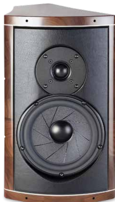
RIGHT: The asymmetric wooden cabinets are 'hand crafted by master artisans' and further braced with aluminium/magnesium alloy sheets. The 29mm Ragnar Lian silk-dome tweeter is joined by a 180mm 'microsphere' bass/mid cone with alloy dust cap
